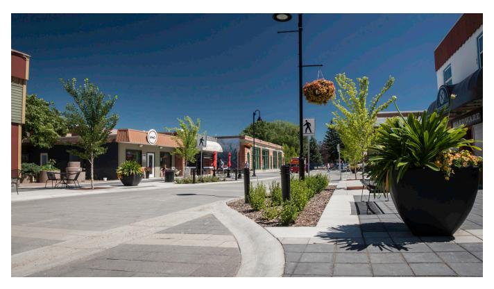
Figure 8: Example of a widened sidewalk with landscaped curb bumpouts, street trees, and street furniture, including planters, benches, and light standards in High River, AB (Photo: O2 Planning + Design).
