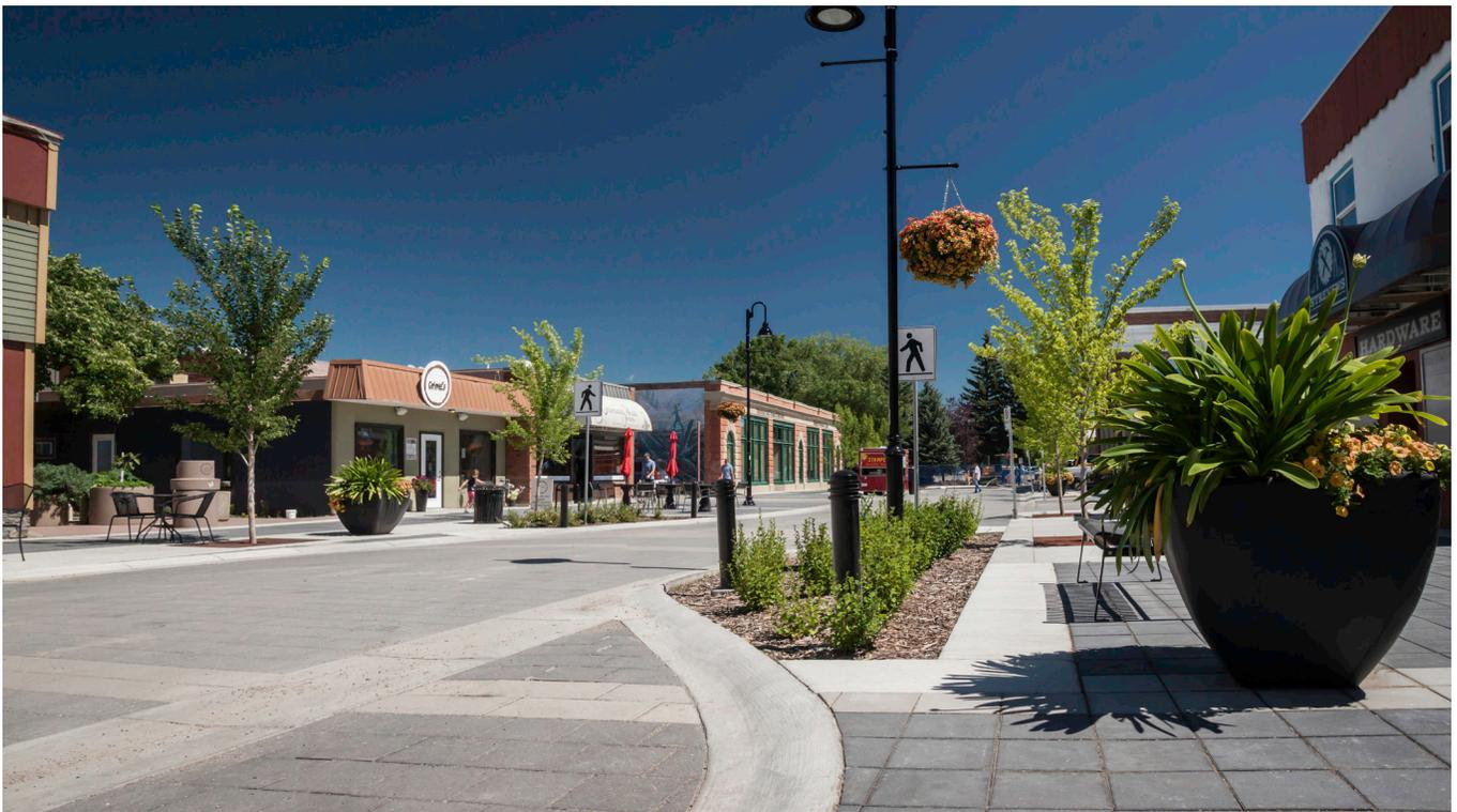
**Figure 8:** Example of a widened sidewalk with landscaped curb bumpouts, street trees, and street furniture, including planters, benches, and light standards in High River, AB (Photo: O2 Planning + Design).
